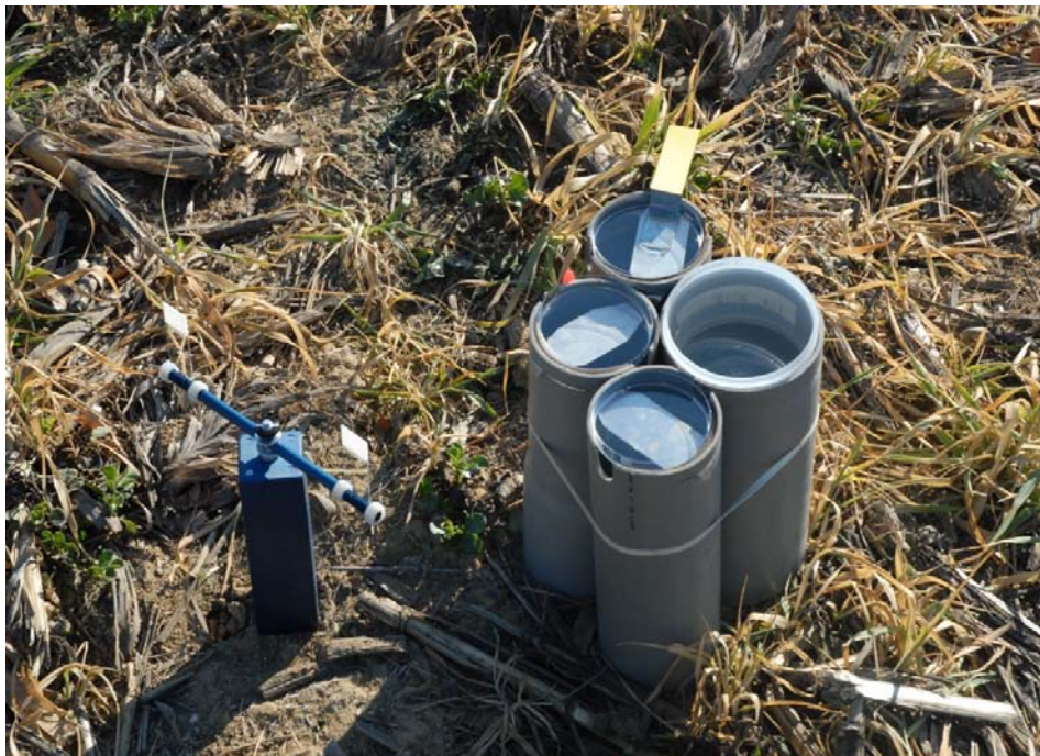
Figure 1: Range of collectors used : (left) Rotary impeger – (right) Petri dishes – Water Sensitive Papers
